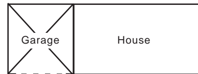
Figure 30 - If the wall of the main house is in line with the wall containing the door of a garage with a room over it, the adjoining wall may help brace the garage.
